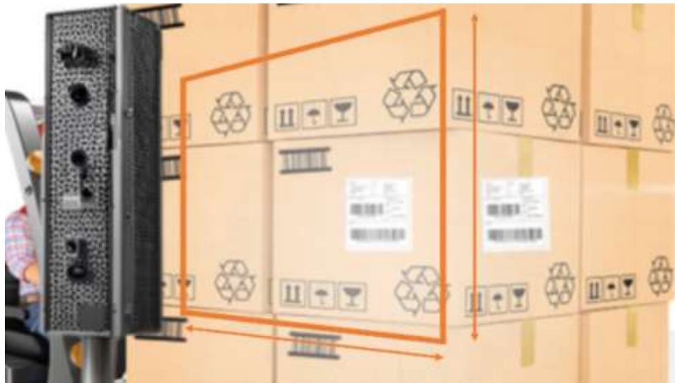
Scanning area depends on the camera and lens FOV
